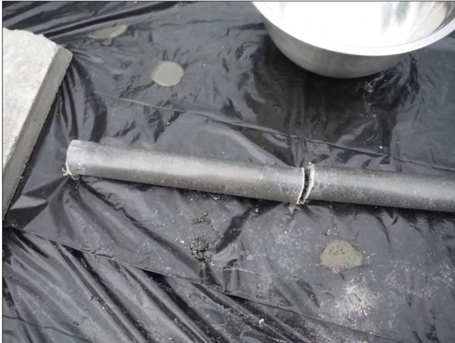
Photo 5: A core barrel filled with sediment after being cut using a hand grinder.
