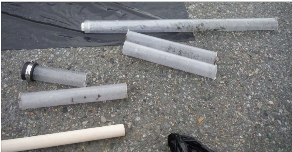
Photo 10: Used core barrels following cutting, soil extrusion and sampling.
