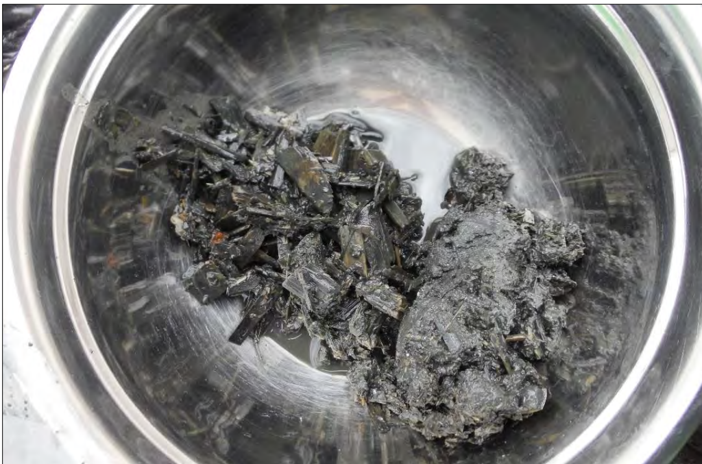
Photo 8: Sediment from location A, consisting of wood waste and soft sediment.
