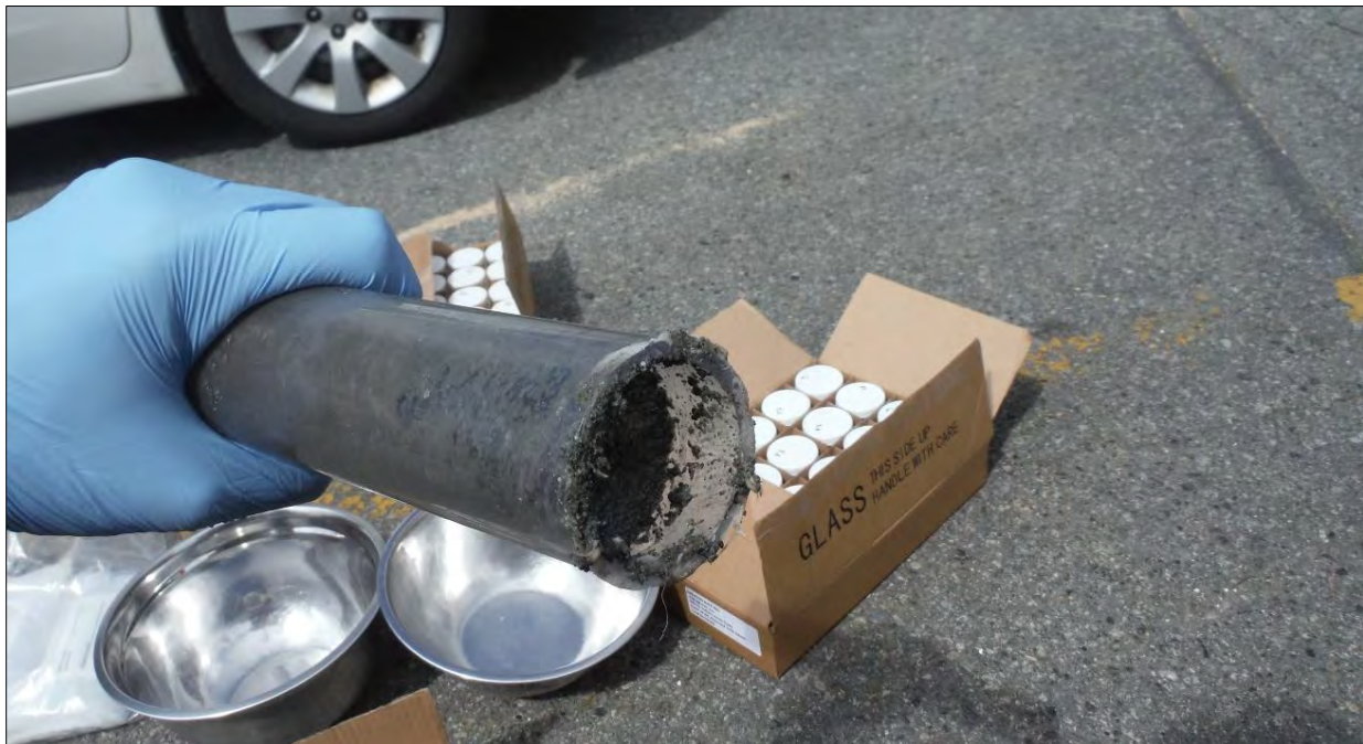
Photo 6: The end of a core section with 2 cm of sediment from the end removed to reduce cross contamination from cutting.
