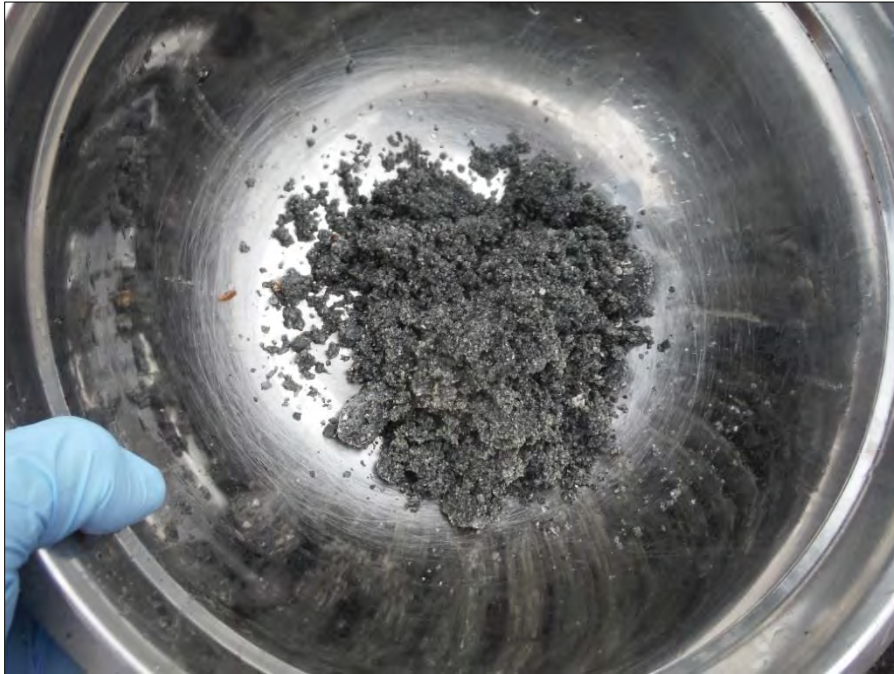
Photo 7: Sediment placed in a bowl from a 30 cm segment of core. Sediment for this section consists of sand, some gravel and shell debris.
