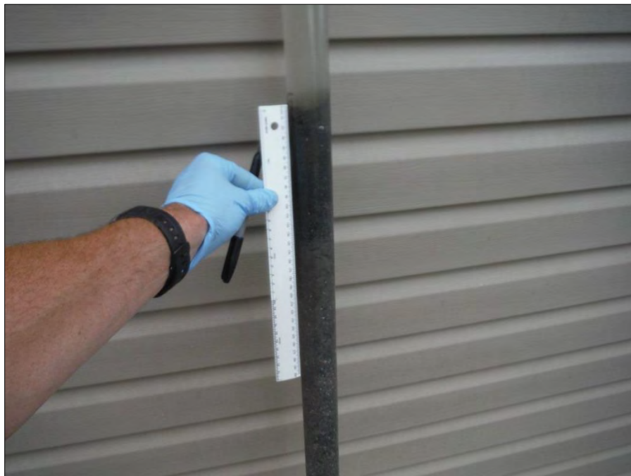
Photo 4: Measuring a core barrel and marking 30 cm intervals.
